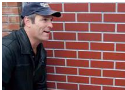
Now for the real test: hurl a 2 x 4 at a precast wall panel at 112 mph. The result: no damage visible, not even a chip.
