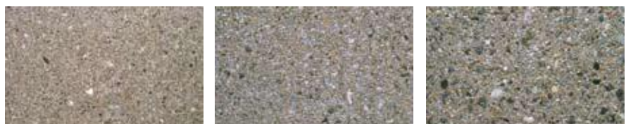
Examples of light, medium, and heavy acid-washed textures.
