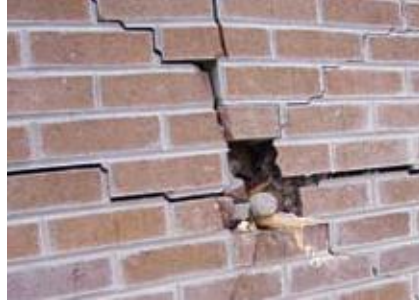
Test two shot the 2 x 4 through a brick wall with wood frame. Surprisingly, it's not all that much safer than siding. What you don't see are the pieces of brick that went flying through the back side of the panel. This wall introduced even more projectiles into the house.
