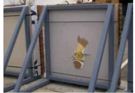
Test three smashed a 2 x 4 through a brick home with steel framing. This damage is still rather significant, but in this test the projectile did not travel through the wall. Looking at the back side shows it would take only slightly more force to push all the way through.
