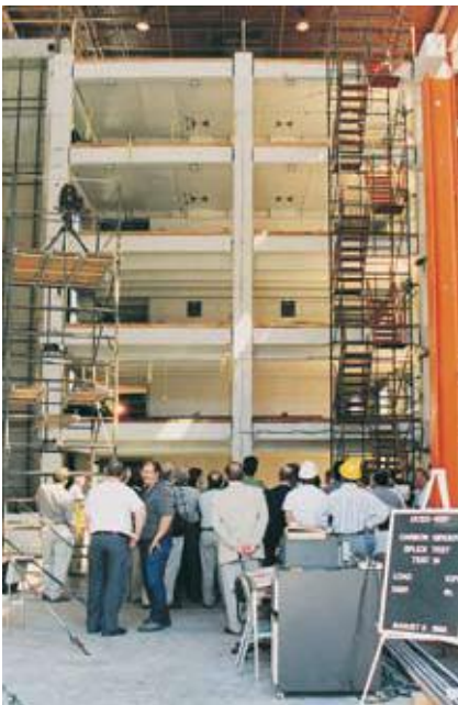
Rigorous tests performed on an experimental structure proved the success of the PRESS program's connection technology.
