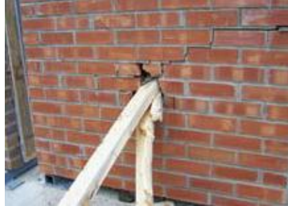
Test three smashed a 2 x 4 through a brick home with steel framing. This damage is still rather significant, but in this test the projectile did not travel through the wall. Looking at the back side shows it would take only slightly more force to push all the way through.
